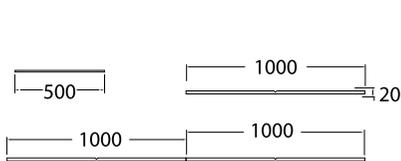
MEDIDA ÚTIL DE LA LÁMINA ACÚSTICA 0.50 M<sup>2</sup>
